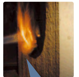
PIR insulation after 30 minutes at over 1000°C
